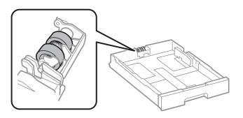
*Important:* Using a dry cloth may damage the surface of the roller.
