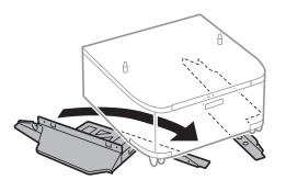
7. Secure the stands with the attachments and screws.
