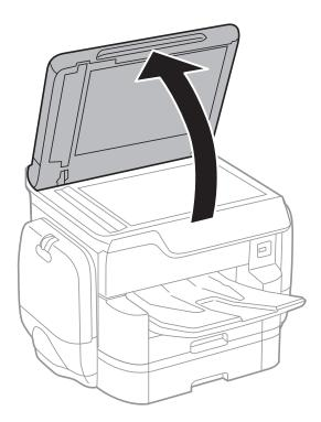
2. Use a soft, dry, clean cloth to clean the surface of the scanner glass.
