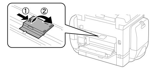
7. Slide out the two used maintenance rollers, and remove them.
