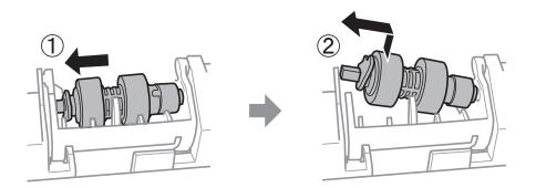
10. Insert the shaft of the new maintenance roller into the hole in the holder, and then slide the shaft on the lever side along the slot while it is facing the flat surface at the front.
