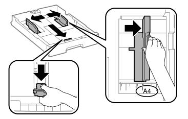
3. Load paper with the printable side facing down, and then slide the front edge guide to the edge of the paper.
