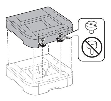
9. Lower the printer gently onto the optional paper cassette aligning the corners, and then secure them with the screws.
