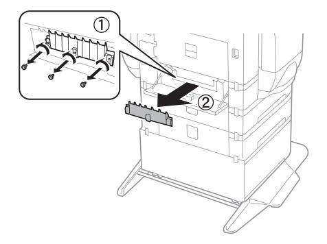
6. Slide out two used maintenance rollers, and remove both of them.
