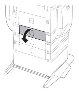
5. Remove the screws by a screwdriver and remove the cover on the rear of inside the printer.
