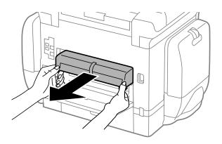
6. Remove the cover inside the back of the printer.
