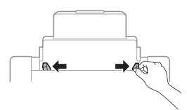
3. Load paper at the center of the rear paper feed with the printable side facing up.
