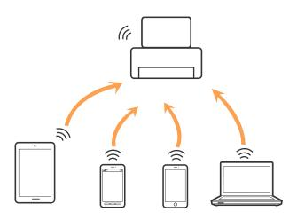
The printer can be connected by Wi-Fi or Ethernet, and Wi-Fi Direct (Simple AP) connection simultaneously. However, if you start a network connection in Wi-Fi Direct (Simple AP) connection when the printer is connected by Wi-Fi, the Wi-Fi is temporarily disconnected.
