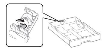
9. Slide the maintenance roller toward the lever, and then remove them by taking the shaft out of the holder.
