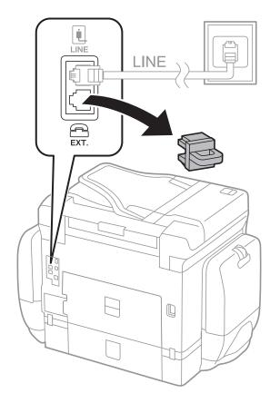
1. Remove the cap from the EXT. port on the back of the printer.
