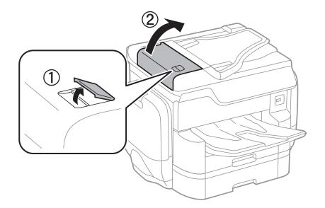
2. Use a soft, moist cloth to clean the roller and the interior of the ADF.
