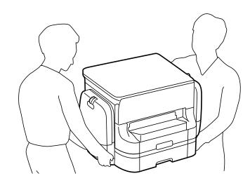
U When carrying the printer, do not tilt it more than 10 degrees; otherwise the printer may fall.
