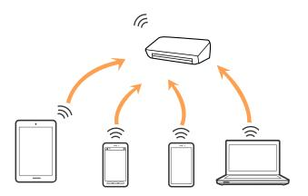
The scanner can be connected by Wi-Fi and Wi-Fi Direct (Simple AP) connection simultaneously. However, if you start a network connection in Wi-Fi Direct (Simple AP) connection when the scanner is connected by Wi-Fi, the Wi-Fi is temporarily disconnected.
