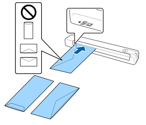
Slide the envelope into the input slot until it meets resistance.
