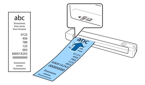
Slide the receipt into the input slot until it meets resistance.
