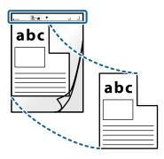
2. Load the Carrier Sheet into the left side of input slot with the top edge facing into the scanner. Slide the Carrier Sheet into the input slot until it meets resistance.
