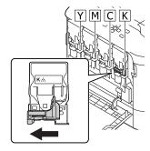
6 Pinch the dents on the cartridge and remove it.
