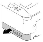
Remove any jammed paper, then close the paper cassette into the printer.
