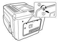
Reattach the rear cover to the printer as shown below.
