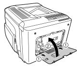
Tighten the screws on the back of the printer.
