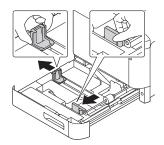
Load a stack of the desired paper on the center of the paper cassette with the printable surface facing up.
