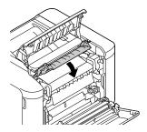
A Lock the release levers on both sides of the fuser unit.
