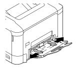
Press down on the center of the paper lifting plate until the left and right locking tabs (white) lock into place.
