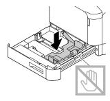
Pinch the knobs and slide the paper guides to accommodate the paper you are loading.
