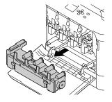
Press "PUSH" on the photoconductor to unlock it and pull it out.
