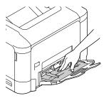
Load a stack of the desired paper with the printable surface facing down.
