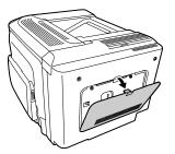
Loosen the two screws on the metal cover that appears, and remove it.
