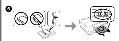
Slide the edge guides to the edges of the paper. Keep the cassette flat and insert it back into the product carefully and slowly.
