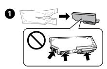
Prepare new ink cartridge(s). Remove the ink cartridge from its package.
