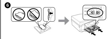
Slide the edge guides to the edges of the paper. Keep the cassette flat and insert it back into the printer carefully and slowly.
