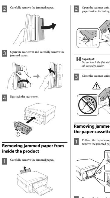
Open the scanner unit. Then remove all of the paper inside, including any torn pieces.
