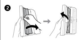
Open the rear cover and carefully remove the jammed paper.
