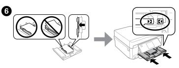
Slide the edge guides to the edges of the paper. Keep the cassette flat and insert it back into the product carefully and slowly.
