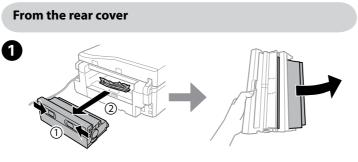
Pull out the rear cover and carefully remove the jammed paper.
