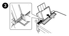
Slide the edge guide against the paper, and flip the guard back.
