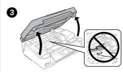
Open the scanner unit and press OK.
