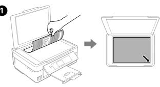
Open the document cover and place your original face-down on the scanner glass. Align the original with the front right corner of the glass.
