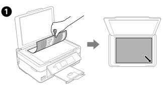
Open the document cover and place your original face-down on the scanner glass. Align the original with the front right corner of the glass.
