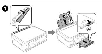
Flip the feeder guard, and then slide out the paper support and the output tray.
