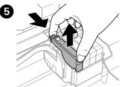
Squeeze the tab on the ink cartridge and lift it out.
