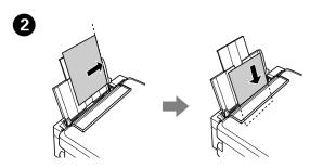
Load paper with the printable side face-up against the right side of the sheet
