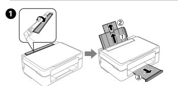
Flip the feeder guard, and then slide out the paper support and the output tray.
