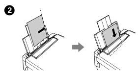
Load paper with the printable side face-up against the right side of the sheet feeder.
