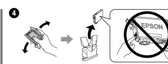
Prepare new ink cartridge(s). For best results, gently shake the new ink cartridge four or five times and then unpack.
