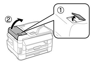
For WF-3620 Series/WF-3640 Series: Open the ADF cover.
