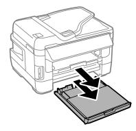
For WF-7610 Series/WF-7620 Series: Remove the cover.
