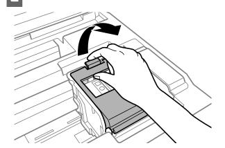
Pinch and remove the ink cartridge.
