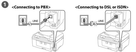
Available phone cable RJ-11 Phone Line / RJ-11 Telephone set connection
