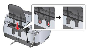
2. Connect the document cover's cable to the TPU interface connector.
