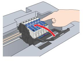
Install all ink cartridges. This product does not work unless all cartridges are installed properly.
