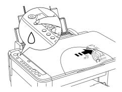
The unit begins charging the ink delivery system. This process takes about one minute to complete. When the ink charging process is finished, The On light stops flashing and remains lit, and the Ink light goes out.
