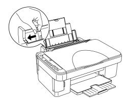
4. Load the paper with the printable side up so it is against the right edge guide, and slide it into the sheet feeder.
