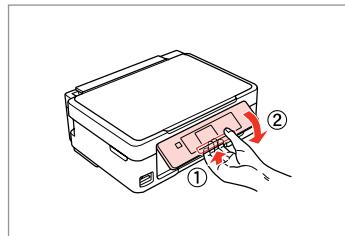
To lower or close the panel, unlock by pulling the lever on the rear until it clicks, and then lower down. Simply lift the panel to raise it.
