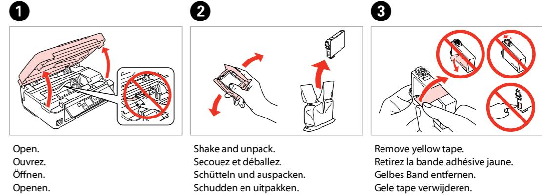
Installing the Ink Cartridges
