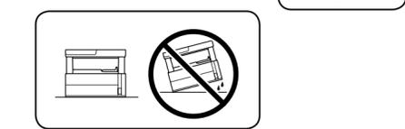
1. Be sure to place the ink bottle upright when tightening the cap. Place the printer and the bottle in a plastic bag separately and keep the printer level as you store and transport it. Otherwise ink may leak. 2. After you move it, remove the tape securing the print head. If you notice a decline in print quality, run a cleaning cycle or align the print head.
