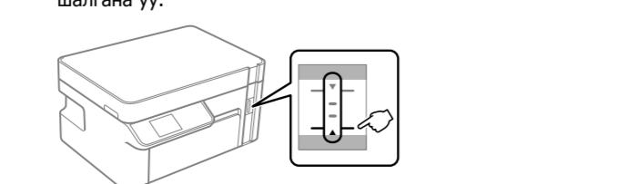
**1** To confirm the actual ink remaining, visually check the ink level of the product's tank. Continued use of the printer when the ink level is below the lower line on the tank could damage the product.
