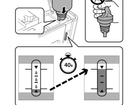
7 Ink starts pouring and the flow stops automatically when the ink reaches the upper line.
