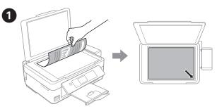
Open the document cover and place your original face-down on the scanner glass. Align the original with the front right corner of the glass.
