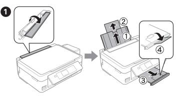
Flip the feeder guard, and then slide out the paper support and the output tray. 翻開進紙槽護蓋,然後滑出紙張支撐板及出紙托盤
