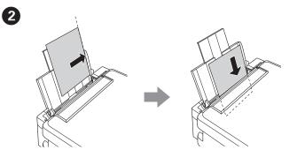
Load paper with the printable side face-up against the right side of the sheet
