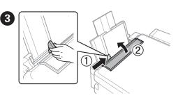
Slide the edge guide against the paper, and flip the guard back. 靠著紙張滑動邊緣定位器,然後翻回護蓋
