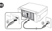
Connect and plug in. 連接電源線並插入電源
