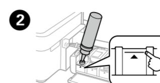
Continuing to use the printer when the ink level is below the lower line will damage the printer. Make sure you visually check the ink levels.
