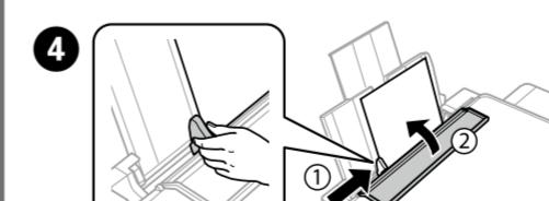
Slide the edge guide against the paper, then close the feeder guard.
