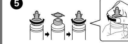
Remove the cap of the ink bottle, remove the seal from the bottle, and then install the cap.
