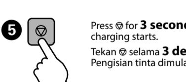
Press for 3 seconds until starts flashing. Ink charging starts.
