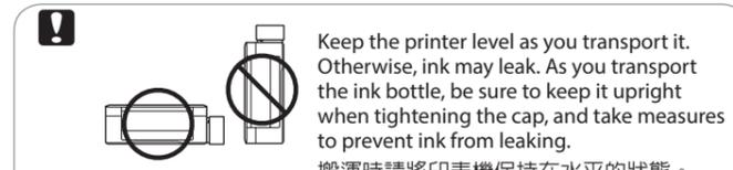
Keep the printer level as you transport it. Otherwise, ink may leak. As you transport the ink bottle, be sure to keep it upright when tightening the cap, and take measures to prevent ink from leaking.
