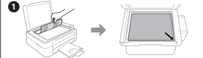
Open the document cover and place your original face-down on the scanner glass. Align the original with the front right corner of the glass.
