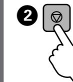
Run print head cleaning until all lines are printed completely. Hold down for 3 seconds until the power light starts flashing. Print head cleaning starts.
