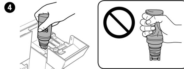
Ink flow stops automatically when the ink level reaches the upper line.
