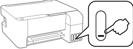
Check the ink levels. If an ink level is below the lower line, refill the ink.
