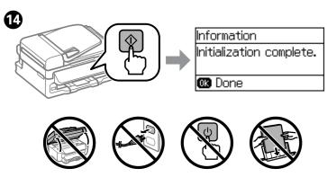
Confirm that the tanks are filled with ink, and then press  $\diamond$  to start charging ink. Charging ink takes about 20 minutes.
