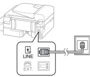
Connect a phone cable to a telephone wall jack and to the LINE port on your product. See the *User's Guide* (PDF) for more details.
