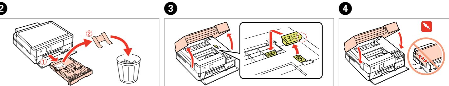
Pull out, remove, and dispose.
