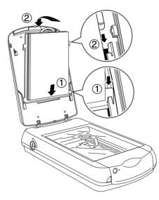
4. Place the document on the document table, with the side to be scanned facing down. Make sure that the document is carefully aligned with in the corner of the document table as shown below.
