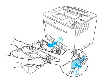
4. Remove the tapes that secure the cassette cover, and then remove the cover. Follow by removing all the tapes and protective materials inside the cassette.
