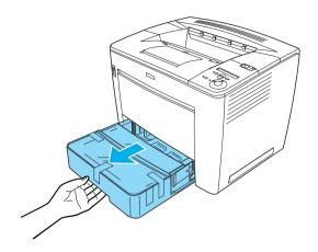
3. While pressing the gray stoppers located on both sides of the paper cassette, pull the cassette out from the printer.
