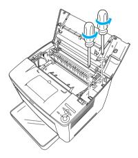
4. Remove the two screws located near the bottom-right edge of the printer.
