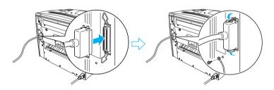
3. Plug the other end of the cable into the computer's USB or parallel interface connector.
