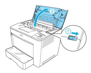
7. Remove the protective materials from inside the printer.
