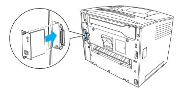
4. Secure the interface card with its screws.
