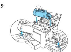
Caution: Do not touch the roller or other parts inside the printer. Doing so may cause the printer to
