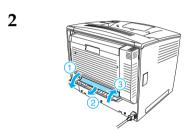
If the paper jam error is not yet cleared, remove the Duplex Unit from the printer. Then check if paper is jammed at the opening on the rear side of the printer.
