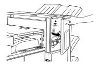
Place one hand under the cartridge. Press the lever down with the other hand, and remove the Staple Cartridge.
