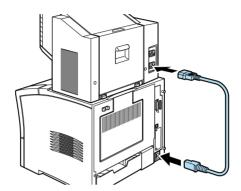
6. Connect the printer's original power cord to the upper power inlet on the Multibin Unit, and plug the other end into an electrical outlet.
