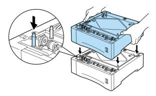
5. Make sure all corners of the upper unit fit securely onto the bottom unit. Remove the paper cassette from the upper unit. Then, insert and tighten the three screws as shown below.
