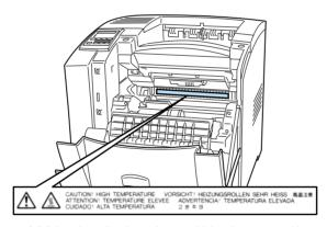
(Visible when the imaging cartridge is removed.)
