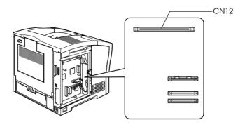
5. Pull the clips on each side of the CN12 outward.
