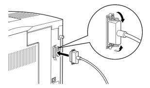
4. Plug the other end of the cable into the computer's parallel interface connector, and fasten it as required.
