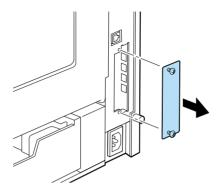
4. With the component side of the optional interface card facing the correct side, slide and push the interface card into the slot as shown below. Push the card firmly to lock it into place.
