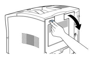
3. Reach into the top rear of the printer and press in on the two plastic tabs locking the top cover in place, while at the same time holding onto the cover so it doesn't fall. Lift the top cover off carefully and store it in a safe place.
