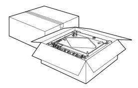
Carefully remove the Large Capacity Paper Unit from its carton and place it on the floor or a flat stable surface. Then, remove the packing tape used to secure the paper cassette in place.
