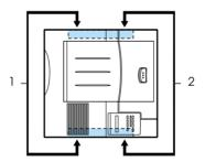
☐ Do not touch the areas inside the front and rear covers of the printer, which are marked with the caution labels. If the printer has been in use, these areas may be very hot.
