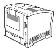
3. Loosen the two retaining screws on the back of the printer and remove the left side casing of the printer.
