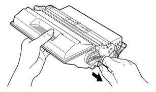
5. Note the arrows on the left and right sides inside the printer. Slide the imaging cartridge, in the direction of the arrows, at a slight downward angle into the printer. Push the cartridge into the printer until it is firmly seated in its proper position.
