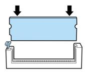
3. Hold the ROM module oriented as shown, then push the ROM module into the slot evenly until the button comes up.
