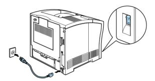
2. Insert the power cord into the AC inlet at the back of the printer. Then plug the other end into a properly grounded electrical outlet.
