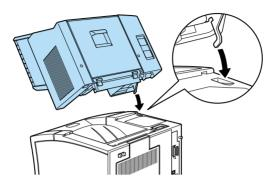
4. Note the location of the interface plug on the Multibin Unit and its counterpart on the printer. Lower the rear of the unit into place and make sure the plug is inserted properly into the receptacle on the printer. Slide the unit slightly as necessary so that the plastic tabs snap into the slot along the rear of the printer.
