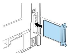
5. Secure the interface card by fastening the two retaining screws.
