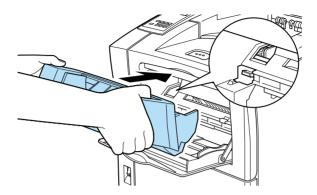
6. Push it straight into position directly above the MP tray.
