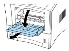
2. Fan a stack of paper and tap it on a flat surface to even the edges. With the printable surface down, load the stack of paper by inserting it all the way into the tray. Then, slide the paper guides against the sides of the paper.
