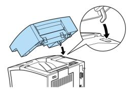
3. Note the location of the interface plug on the Shifter and its counterpart on the printer. Lower the rear of the unit into place and make sure the plug is inserted properly into the receptacle on the printer. Slide the unit slightly as necessary so that the plastic tabs snap into the slot along the rear of the printer.
