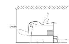
When installing the Optional 250-Sheet Lower Paper Cassette Unit, the space for placing the printer needs 10.6 cm additional height.
