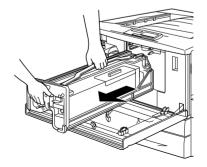
7. Take the new photoconductor unit out of its package and unwrap the protective sheet while holding the handle as shown below.
