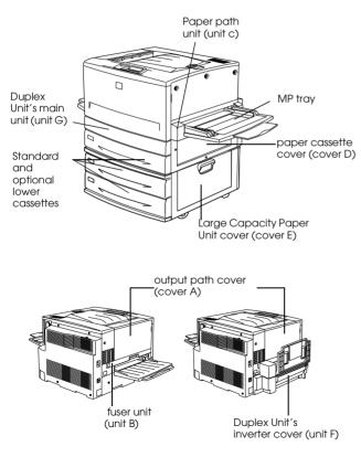
If a paper jam occurs at two or more locations simultaneously, the corresponding multiple locations are displayed.
