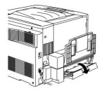
2. Gently remove the jammed paper inside the inverter cover.
