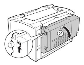
4. Open the paper holder by pulling down the lever with a black star on it.
