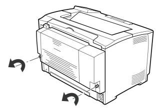
3. Press the unlock button to unlock the hooks, then remove the Duplex Unit from the printer.
