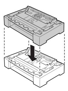
6. Secure the optional paper cassette units with the four fittings. Install two of the four fittings inside on both sides of the optional paper cassette unit and the other two fittings outside on both sides.
