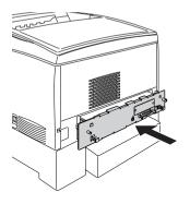
2. Fasten the circuit board tray with the two screws.
