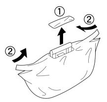
4. Unwrap the protective sheet and material while holding the handle as shown below.
