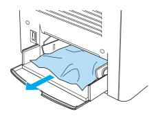
5. Remove paper stacked on the MP tray. Check if any paper is jammed inside the MP tray.
