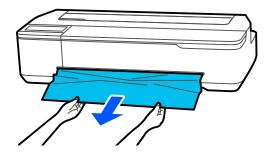
6 Open the front cover, remove the jammed paper, then close the front cover.
