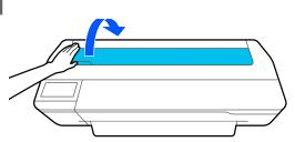
3 Load a sheet of paper with the print side facing up, and then align its right edge with the mark line on the right and its left edge with the mark line for the paper size.
