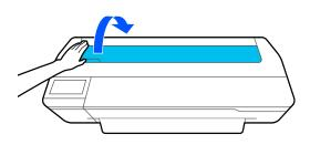
Tilt the auto sheet feeder toward the back and then pull it out upward.
