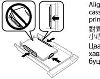
Align the edges of the paper. Keep the cassette flat and insert it back into the printer carefully and slowly.
