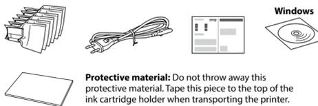
**Protective material:** Do not throw away this protective material. Tape this piece to the top of the ink cartridge holder when transporting the printer.
