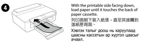
4 With the printable side facing down, load paper until it touches the back of paper cassette.
