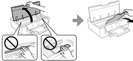
Open the printer cover, and then remove the jammed paper carefully.
