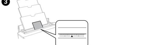
3 Load paper at the center ▲ mark of the rear paper feed with the printable side facing up.
