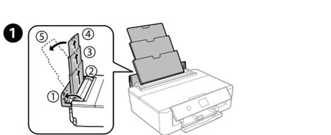
1 Open the feeder guard, extend the paper support, and then tilt it backwards.
