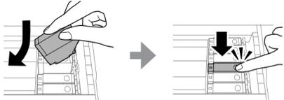
Insert the ink cartridge diagonally into the cartridge holder and gently push it down until it clicks into place.
