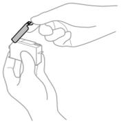
Remove the cap from the new cartridge.
