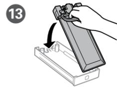
Fit the ink supply unit into the ink supply unit tray.
