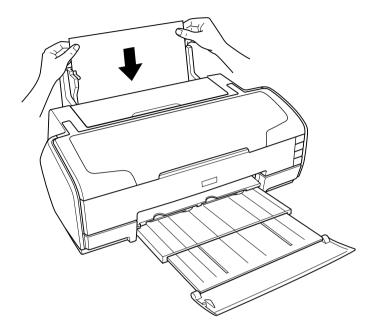
Insert the paper into the rear manual feed slot until the paper meets resistance. Maintain a constant pressure against the paper until you feel the printer pull the paper in slightly. Let go of the paper to allow the printer to adjust the paper position.
