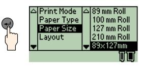
Press the  $\blacktriangledown$  button to highlight 100 mm  $\times$  150 mm, then press the - Select button.
