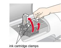
Do not move the print head by hand, as this may damage the
