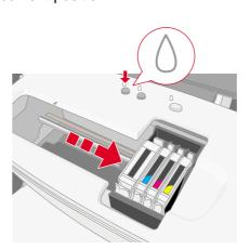
4. Install the new ink cartridges as explained on the Setup in the "Install the ink cartridges" section.
