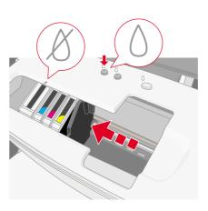
3. Then, press the ∆ ink button again. The print head moves to the ink cartridge replacement position.
