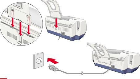
If the printer comes on when you plug in the power cord, turn off the printer by holding down the  $\circ$  power button until the light goes out.
