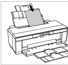
Load the paper with the printable side up.
