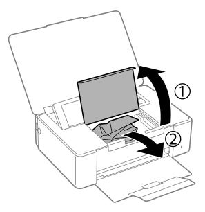
Check that there is no paper remaining in the printer, and then close the inner cover.
