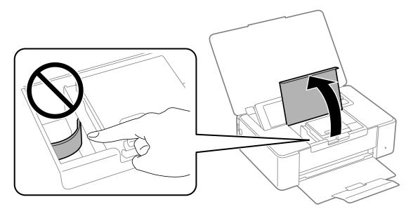
Push the tab to unlock the ink cartridge holder, and then remove the cartridge diagonally.
