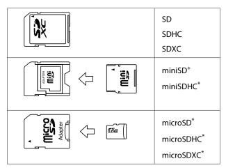
\* Attach an adapter to fit the memory card slot. Otherwise, the card may get stuck.
