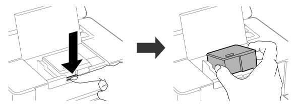
Insert the ink cartridge diagonally into the cartridge holder and gently push it down until it clicks into place.
