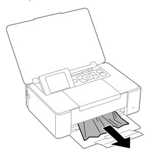
If you still cannot remove the paper, open the inner cover to remove it.
