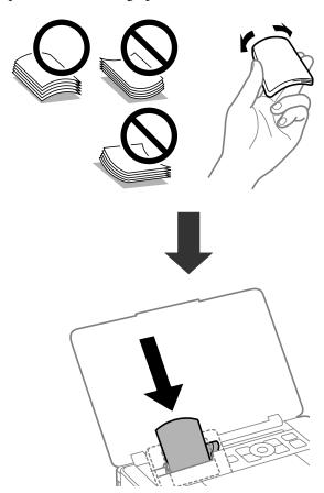
☐ Fan and align the edges of the envelopes before loading. When the stacked envelopes are puffed up with air, press them down to flatten them before loading.
