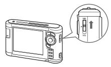
To release Hold, slide the power switch back to the middle.
