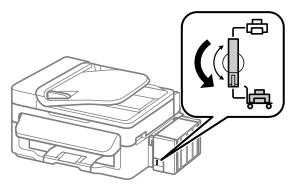
Unhook the ink tank unit from the product and lay it down, and then make sure to install the cap onto the ink tank securely.
