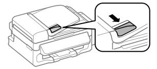
Insert the originals face-up and short edge first into the Automatic Document Feeder.
