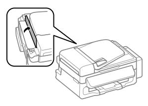
Slide out the paper support and the output tray and then raise the stopper.
