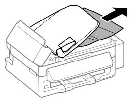
Return the ADF input tray to its original position, and close the ADF cover.
