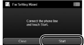
When the fax setting wizard screen is displayed, tap start to configure the minimum settings for fax features. If you do not want to configure them now, close the fax setting screen. The home screen is displayed and printer is ready for printing.
